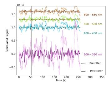
**Figure 5.** Corrected signal,  $D_{i,est}(t)$  for the Almost Limb activity 1969A, after spectral filtering has been applied to each wavelength range (solid lines) compared with the original data (dashed lines). The vertical black line on the plot, denotes the time  $(t_v)$  when the telescope's line of view hits the Moon's surface. An offset has been added here too to view each wavelength range distinctly. Note the filtered data shows much smaller fluctuations than the raw data.
