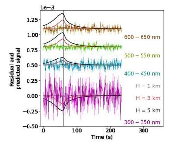
**Figure B2.** This figure shows the filtered residual signal for "1918A," for each wavelength range. The signal predicted using the Fraunhofer model and the exponential density profile is plotted over the residual signal for a scale heights of 1, 3, and 5 km in gray, lightcoral, and black, respectively. An offset has been added to view the signals distinctly.
