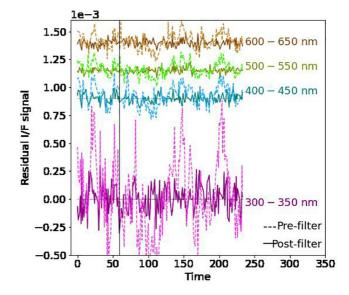
**Figure B1.** Corrected signal (in solid) for the set "1918A," after spectral filtering has been applied to each wavelength range and the original spectrum (in dotted), plotted against time. An offset has been added here too to view each wavelength range distinctly.
