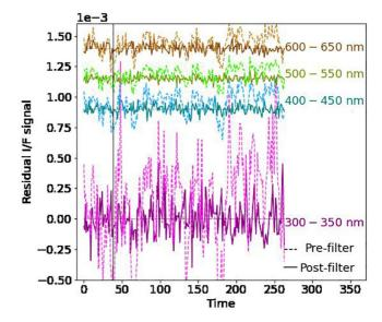
**Figure B3.** Corrected signal (in solid) for the set "1929A", after spectral filtering has been applied to each wavelength range and the original spectrum (in dotted), plotted against time. An offset has been added here too to view each wavelength range distinctly.
