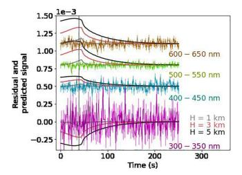
**Figure B6.** This figure shows the filtered residual signal for "1956A" for each wavelength range. The signal predicted using the Fraunhofer model and the exponential density profile is plotted over the residual signal for a scale heights of 1, 3, and 5 km in gray, lightcoral respectively. An offset has been added to view the signals distinctly.
