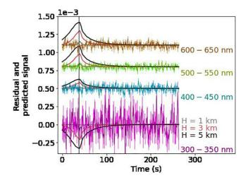
**Figure B4.** This figure shows the filtered residual signal for "1929A" for each wavelength range. The signal predicted using the Fraunhofer model and the exponential density profile is plotted over the residual signal for a scale heights of 1, 3, and 5 km in gray, lightcoral and black respectively. An offset has been added to view the signals distinctly.
