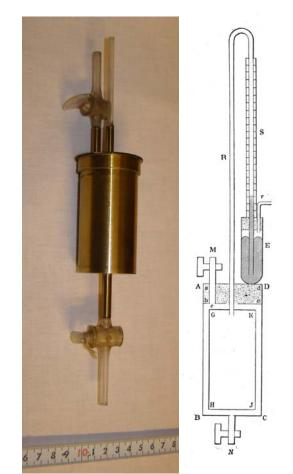
Figure 3. (Left) Picture of the diathermometer used by Stefan to make thermal conductivity measurements of gases (Photo by the author). (Right) Schematic of the diathermometer. The gas is bled into the cavity e through valve M, between concentric cylinders ABCD and GHJK. The cylinders are then placed in a temperature bath and the change of pressure is measured as a function of time (Courtesy of the Austrian Academy of Sciences).
