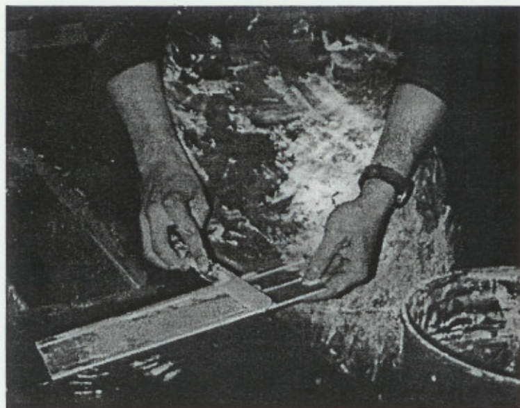
Figure 5. Application of simulated corrosion product to the mock aluminum plate fuel elements.
