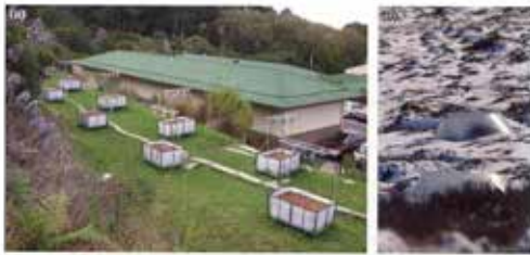
FIGURE 10.9 Active (a) and Passive (b) Warming Experiments. The active warming devices include the use of infrared warming lamps. Passive warming depends on blocking of air circulation or intensification of sunlight to create warmth. Passive warming devices are often simply circles or boxes of glass or clear plastic, which act much like miniature greenhouses but allow multispecies interactions and have minimal impact on nocturnal precipitation. (a) Courtesy of Charles Must. (b) From the National Center for Ecological Analysis and Synthesis, University of California, Santa Barbara.
