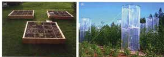
FIGURE 10.10 Transplantation and Open-top Chamber Experiments. Transplantation preserves plant-plant interactions and soil properties. It is usually implemented with the movement of plants embedded in whole soil. Open-top chambers preserve plant and soil relationships over a limited area. Source: Finnish Forest Research Institute.
