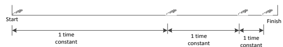
Figure 8.10. Time constant of a first order system. In each time constant, the frog is 63% closer.
