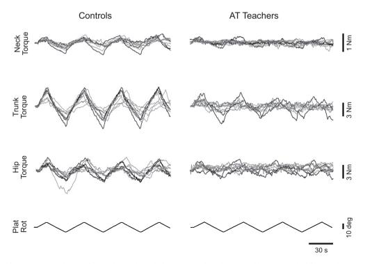
**Fig. 2.** Torsional resistance of AT teachers and matched controls. Single neck, trunk and hip trials overlaid from 9 subjects (6 female, gray lines; 3 male, black lines) from each group. Upwards Plat Rot deflection indicates CCW platform rotation; upwards Torque deflection indicates resistance to CCW rotation.
