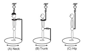
**Fig. 1.** Three configurations of the twisting apparatus. Subjects stood on a platform that rotates the feet and lower segment together while the upper segment is fixed above to a rigid frame, via a suspension system (zigzag lines) and torque sensor (T). (A) Neck: shoulders affixed to the rotating platform with head fixed above. (B) Trunk: pelvis affixed to rotating platform with shoulders fixed above. (C) Hip: feet rotated with platform with pelvis fixed above.
