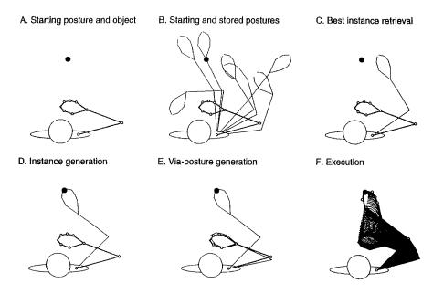
*Figure 1.* Overview of the grasping model. A: Stick figure with nine movable joints and object to be grasped (closed circle). B: Starting posture as in first panel plus seven stored postures. C: Best retrieved instance (most suitable stored posture) for current task. D: New posture identified through instance generation. E: Via posture (posture near original starting posture) that permits most effective collision-free movement. F: Execution (movement).
