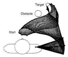
Figure 11. Example of a simulated reach-and-grasp movement performed in the presence of an intermediate obstacle.
