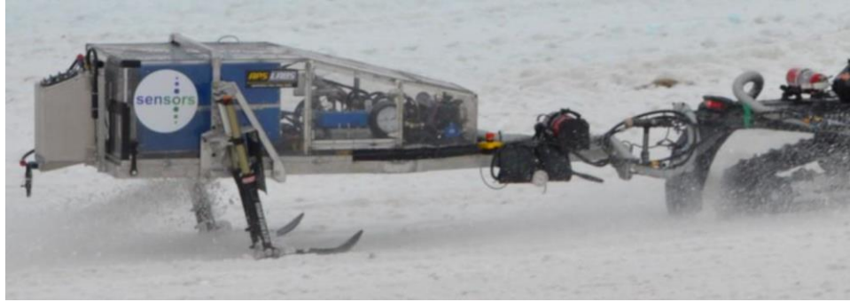
Figure 1: Emissions Tow-Behind at SAE Clean Snowmobile Competition taken by UICSC during 2022 competition.
