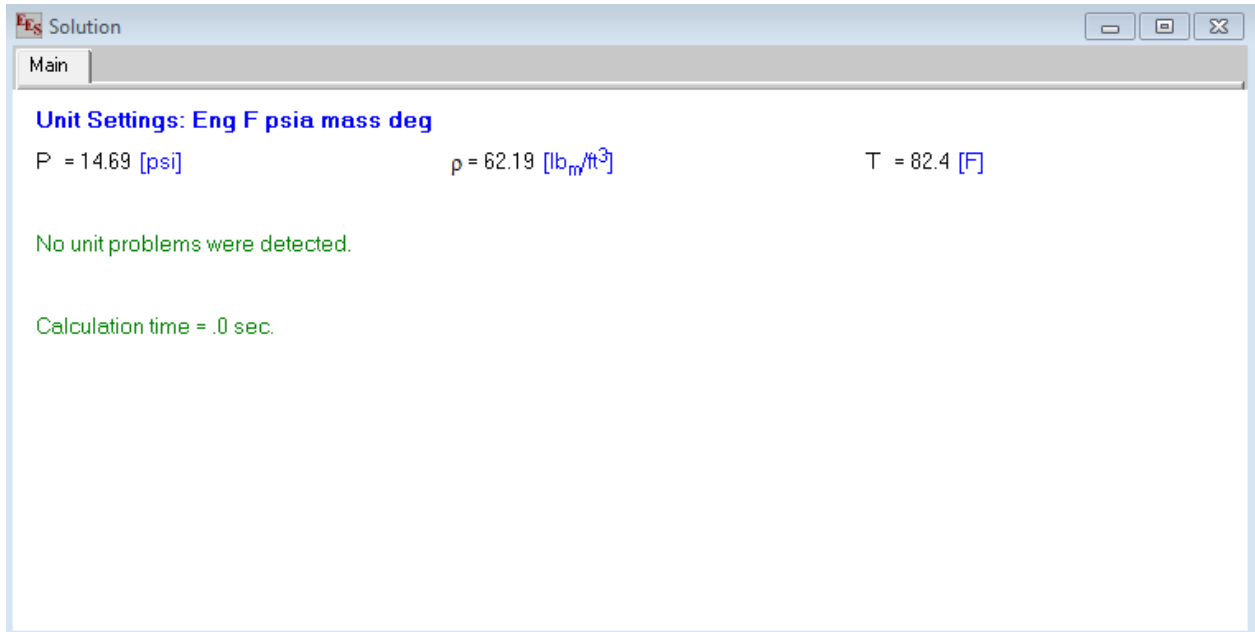
Figure 1: Solutions screen with correct units. Notice “no unit problems detected” labeled at the bottom of the screen.
