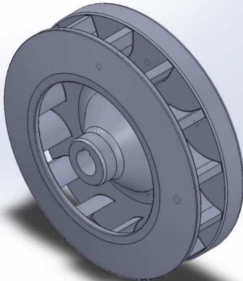
Here is a screen capture of the final part. The hole threads can be seen through the part because I checked the cosmetic thread checkbox. After this I modified the material to be Alloy Steel.
