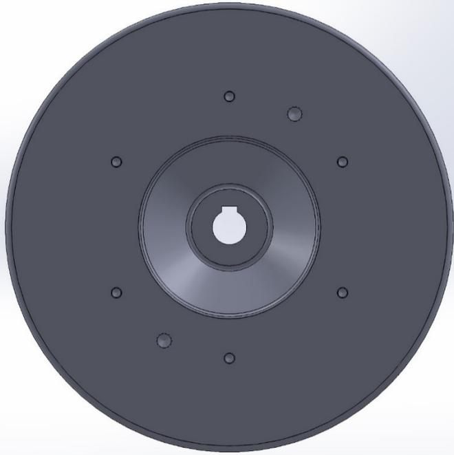
The two M10 Holes were also made using hole wizard and then placed opposite each other. I assumed the holes were equidistant from the M7 holes around them.
