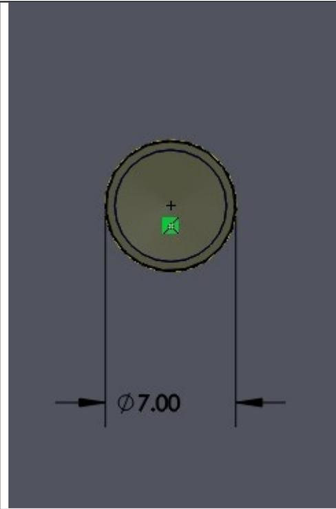
In order to create the M7 hole pattern I used the hole wizard to make one hole and a cut extrude to remove the first 2mm of thread then circular patterned both features.
