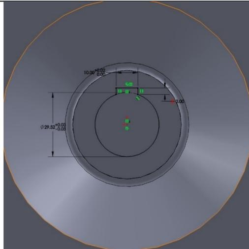
To create the cut through the center of the part for the shaft and keyway I used a lofted cut. Two sketches were drawn, one on the top face and one underneath. The circles have the defined diameters from the drawing to create the appropriate conicity.
