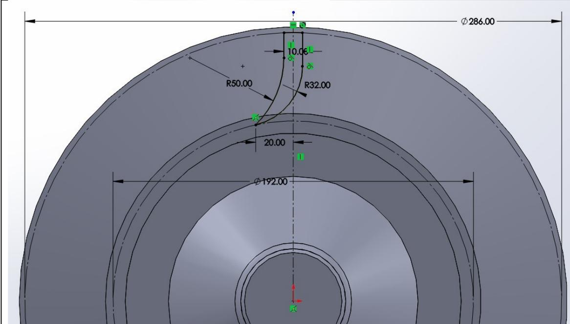
The next sketch was to create one fin which could be circular patterned. I sketched on the face of the lower disk. The outside edge of the fin was defined using a 286mm circle and then two vertical lines were brought down off of the circle. Two tangent arcs were added at the end of the lines and then connected into a point on the other end. Using the given dimension of 192mm the end point was constrained. Then the two arc radii and width dimensions were added, fully defining the sketch.
