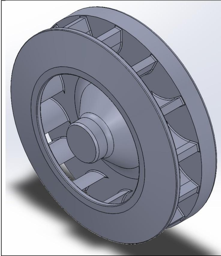
The next feature was adding fillets to the edges of the upper ring. Based on the drawing, I assumed all of the fillets were the same and added 1mm fillets to all of the edges.
